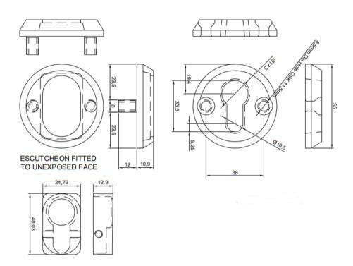
The SEU1090.2. Security escutcheon which was fitted to both doorsets included within WF report No 341512 was not fitted with any intumescent material.
