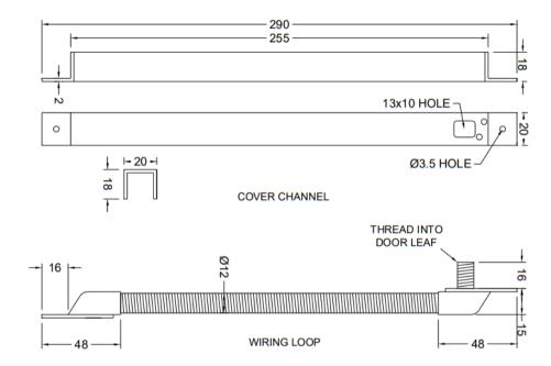
The ALP101 Door Loop which the main body was fitted to the door frame on both doorsets included within WF report No 341512 and was wrapped in a 2 mm layer of Interdens intumescent sheet, this was applied to the outer channel on all sides, was also applied below and behind the end cap that was inserted into the door leaf. This forms the minimum level of intumescent protection required for the ASEL2460 Electric Lock.
