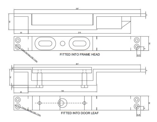
The AEMSF300 Shear Electro-magnetic Lock which was fitted to both doorsets included within WF report No 341512 and was wrapped in a 2 mm layer of Interdens intumescent sheet, this was applied to all parts that where morticed into the door frame and door leaf. This forms the minimum level of intumescent protection required for the AEMSF300 Shear Electro-magnetic Lock.
