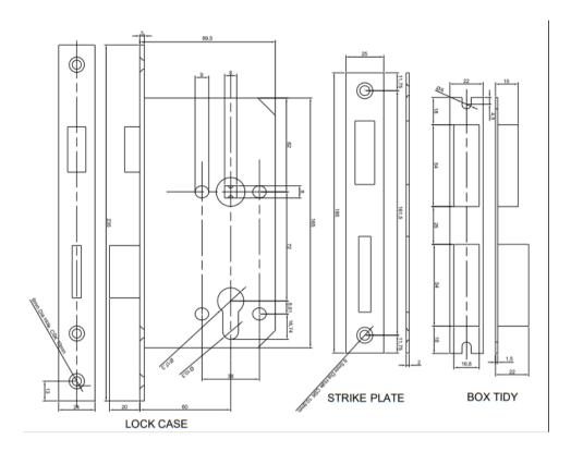
The ASEL2460 Electric Lock which was fitted to both doorsets included within WF report No 341512 and was wrapped in a 2 mm layer of Interdens intumescent sheet, this was applied to all sides of the lockcase and behind the forend plate, this was also applied to the rear of the strikeplate. This forms the minimum level of intumescent protection required for the ASEL2460 Electric Lock.
